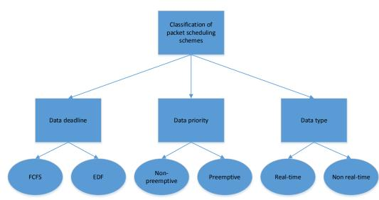
Fig. 2: Classification of packet scheduling schemesDeadline: Packet scheduling schemes can be classified based on the deadline of the arrival of data packets to the base station (BS)
