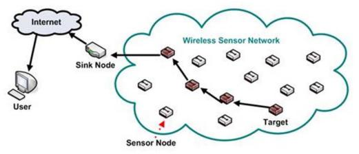
Fig. 1: Network model of wireless sensor network
